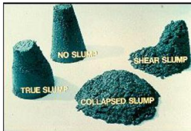
Figure 10 Different possible slump test results.
